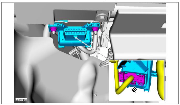
8. Connect the T-harness to the gateway module electrical connector.
